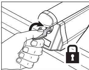
(EN) Rotate the key clockwise bringing it to the vertical position in order to block the cap.
