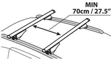
(EN) Ensure that the bar is perfectly centered by checking the extremities from the front and the rear of the vehicle.
