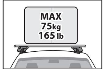
(EN) Do not exceed the maximum load specified for the roof rack, accessory rack or the maximum load recommended by the vehicle manufacturer. **Max roof load = weight of the complete roof rack system + weight of the load**
