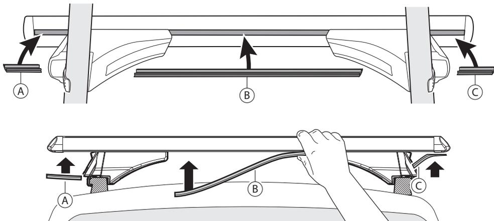
(EN) In case of whistling while driving, in order to reduce such noise, slightly move both bars toward the rear of the vehicle, keeping a minimum distance of 70cm - 27.5" between the two crossbars.
