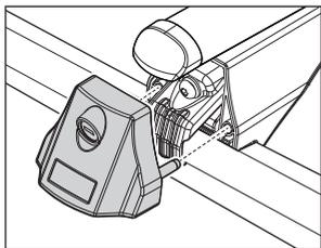
(EN) Install each cap on one jaw and ensure that the key is in the horizontal position.
